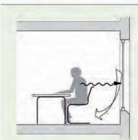
▲ Figure 13 Cold radiation and downdraughts are reduced by the use of low-e coatings thereby increasing comfort as well as reducing heat loss
